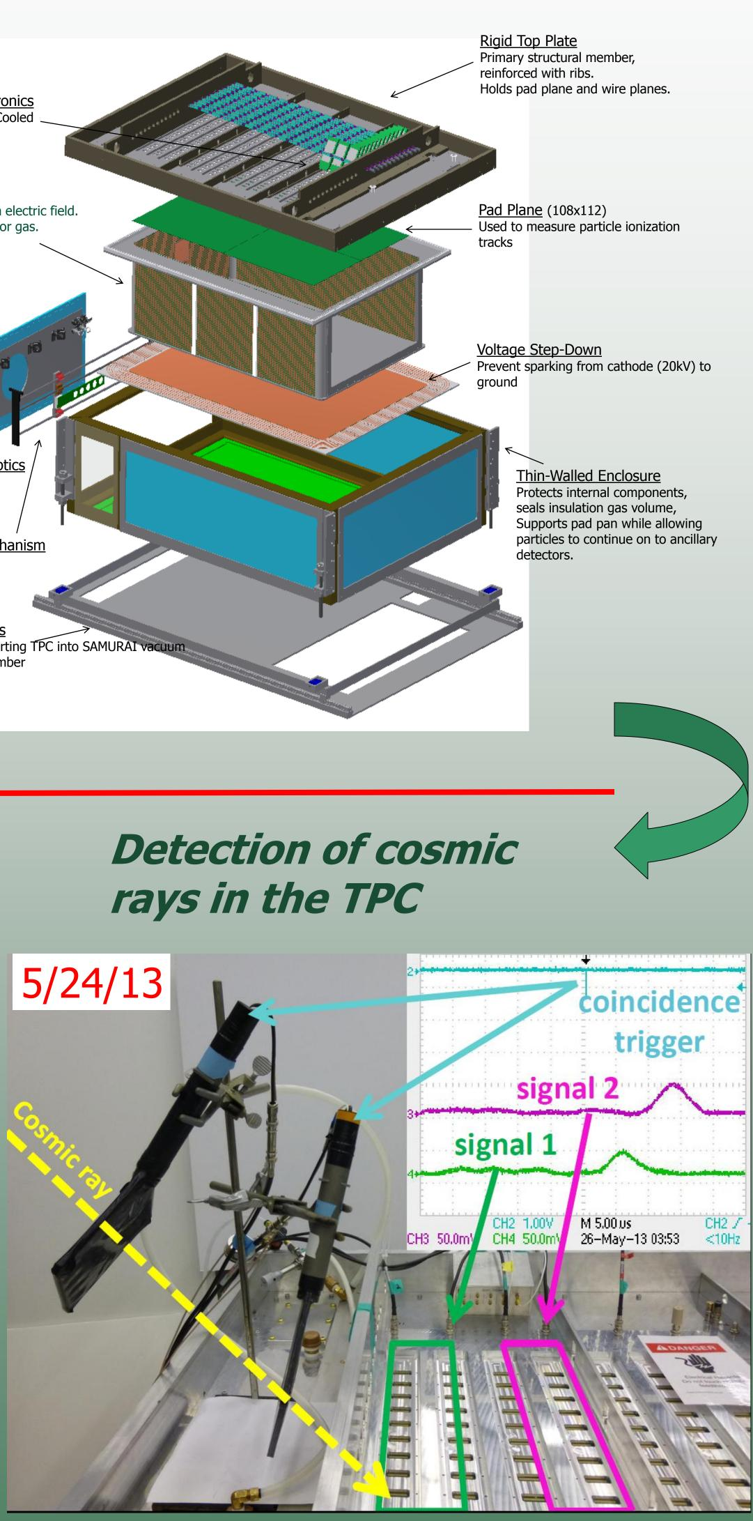
Cosmic rays passing through two scintillator paddles will pass through the sTPC. We use the coincidence signals in the two paddles as triggers for DAQ. The recorded events are then analyzed to reconstruct the tracks.
