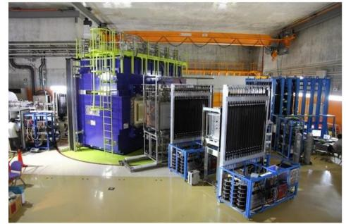
•Charged fragments from collisions ionise the gas along their trajectories •Field cage defines a uniform electric field which drifts ionisation electrons
